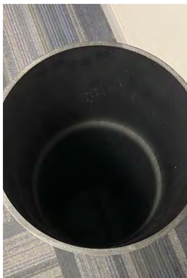
The ducting has a diameter of 225mm
