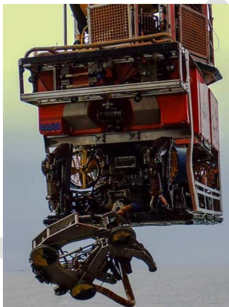
Figure 7-10: Diamond wire cutting tool deployed from an ROV 19
