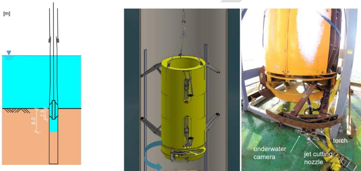
Figure 7-7: Internal water jet cutting 16
