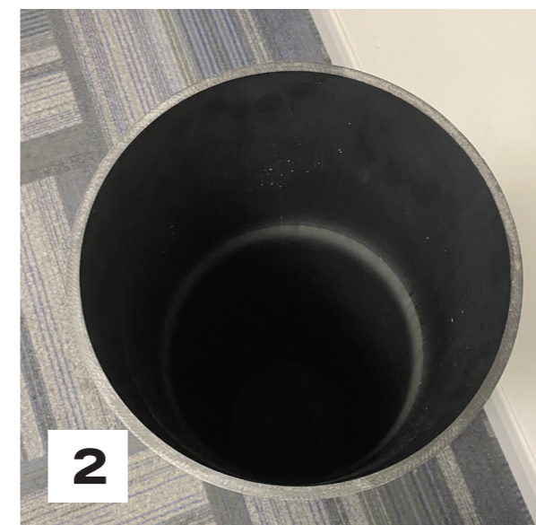
IMAGE 2 - THE DUCTING HAS A DIAMETER OF 225MM
